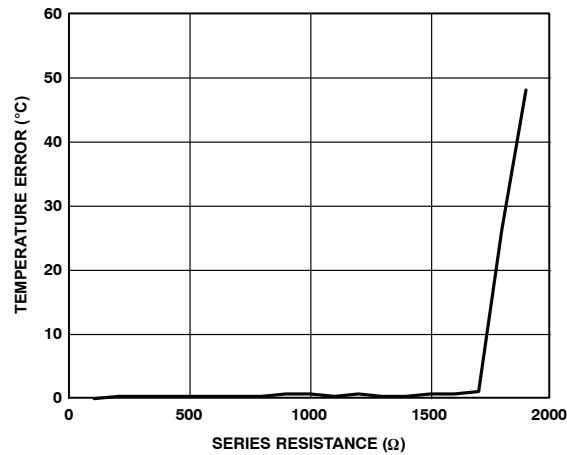
Figure 13. Temperature Error vs. Series Resistance
