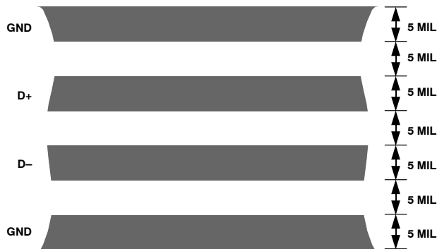
Figure 22. Typical Arrangement of Signal Tracks
